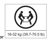
The weight of this part or unit is between 18 and 32 kg (39.7 and 70.5 lb). It takes two persons to safely lift this part or unit. (C009)
